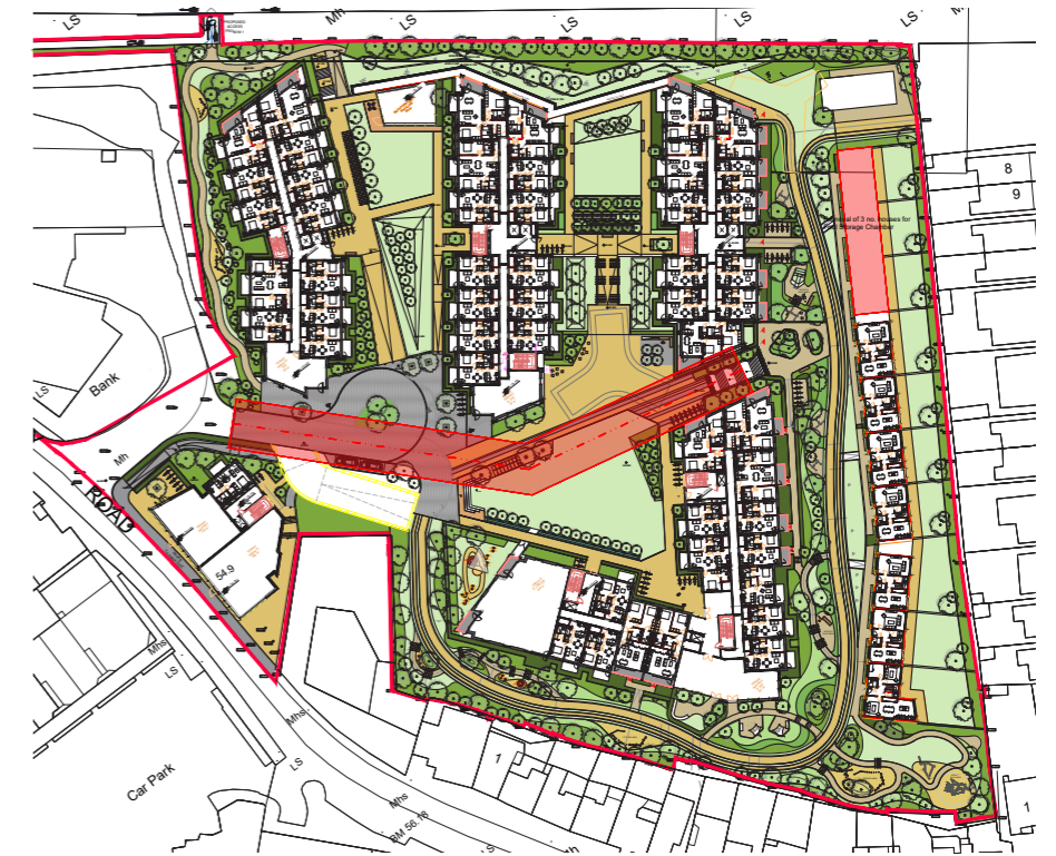
Proposed Route for Irish Water Pipe Overlaid onto Site Layout
